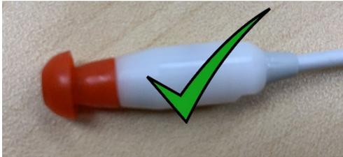
After selecting an eartip, push it onto the probe tube until it is flush against the base of the probe tube. Twisting the eartip slightly while pushing it onto the probe tube is recommended. Be sure the eartip is fully seated on the probe.
