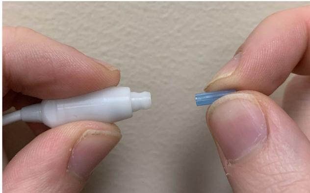
A properly inserted probe tube will snap securely into place when it is fully seated in the probe head.
