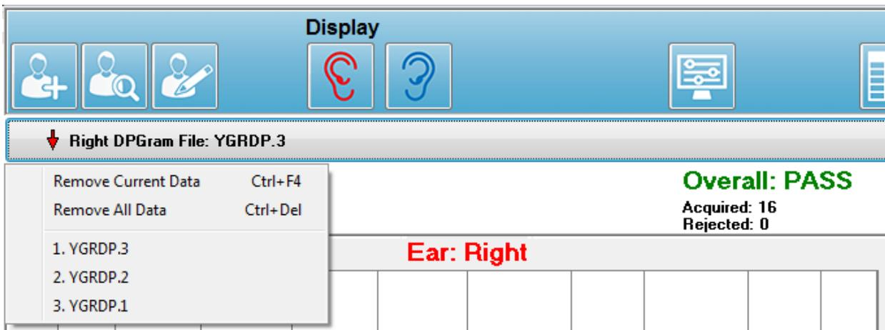
The button is labeled with the ear and filename currently being displayed. Selecting the button presents a dropdown menu. Options for removing the current record or all records are followed by the list of loaded recordings. Click on any loaded record to display on the DPGram. Display options can show the other records as lines on the DPGram.
