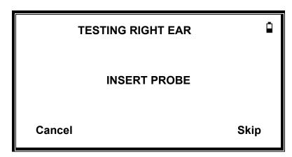
Press ► to skip testing of the right ear and view results for the left ear. Press ◀ to return to the main menu.
