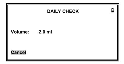
Remove the probe and repeat the test with the three remaining test cavities. The display should show the volume of the 0.2ml, & 0.5ml test cavities to within  $\pm$  0.1ml. The volume of the 5.0ml test cavity should be shown within  $\pm$  0.25ml. When the checks have been completed press  $\triangleleft$  to return to main menu.
