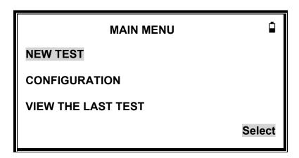
A battery state indicator is shown in the top right corner of the display (except when showing test results). This shows the battery state as a progressively emptying battery. The battery-pack should be recharged when the symbol has a "!" in front of it, or when advised to do so when the instrument is switched on.
