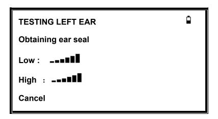
The number of bars shown indicates the robustness of the seal. The probe should be adjusted in the ear until two or more bars are shown for Low and High.
