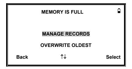
Selecting MANAGE RECORDS will display the DATA MANAGEMENT menu which provides options for printing or transferring data to a computer prior to deleting records to make space for the new test.
