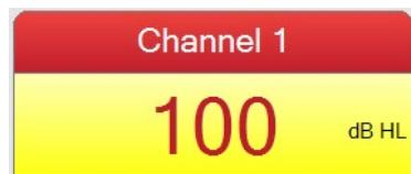
The Pello audiometer is capable of outputting loud sounds and is designed to provide a visual indicator to the examiner when presenting sounds at or above 100 dB. The level display is shown with a yellow background when loud output is selected for presentation.
