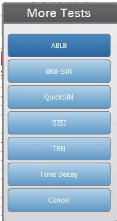
Pressing the “More” test type button calls up a menu of the following special tests if the Special Test and/or Speech Plus license has been installed: ABLB, BKB-SIN, QuickSIN, SISI, TEN, and Tone Decay. Use the on-board navigation buttons or an external mouse to select the special test.
