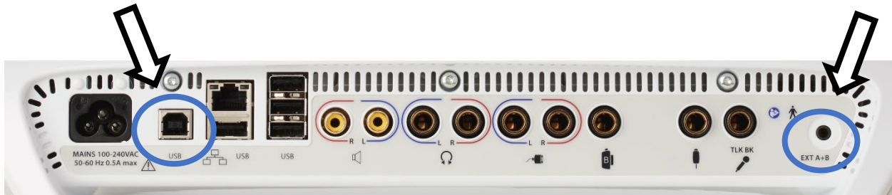
Pello rear panel – USB and External Input ports
