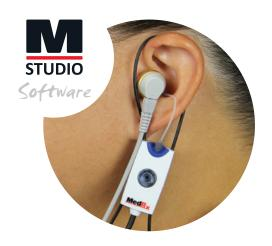
Measure the ear response with an ear tip or ear mold
