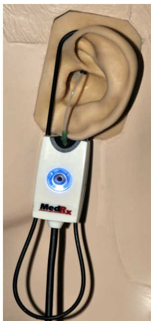
Probe Tube Insertion Guide for Live Speech Mapping and Conventional REM (re: Pomford, J & Sinclair, S. Real-Ear Measurement: Basic Terminology and Procedures. Audiology OnLine.com)
