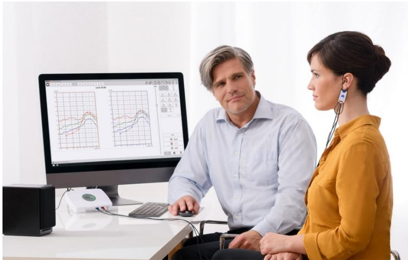
The AVANT REM+ is a device that is used in measuring the real ear acoustical characteristics of hearing instruments in-situ. The device performs measurements of real ear acoustical characteristics of a hearing instrument on a given human ear, and does comply with the International Standards ANSI S-3.46 and IEC 61669.
