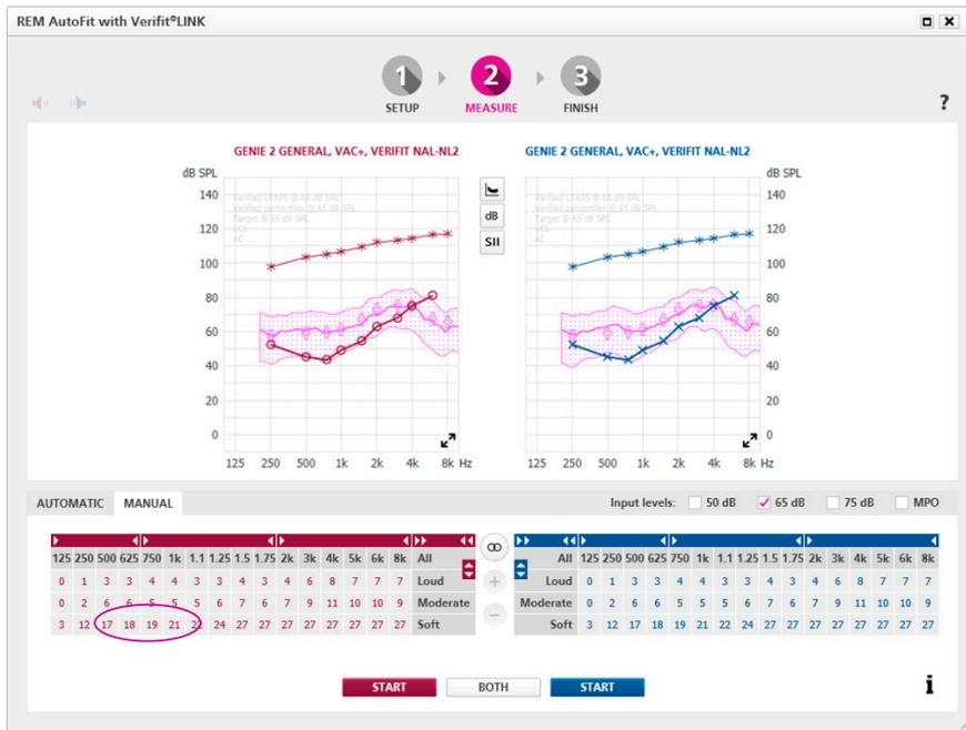
**Manual:** lets you fine-tune the instrument gain to get even closer to target or to personalize the fitting based on your client's comments. This manual process can be done after or instead of the automatic process. Within the REM AutoFit tool, use the fine-tuning controls to adjust the gain and then manually run a measurement to verify the target match.
