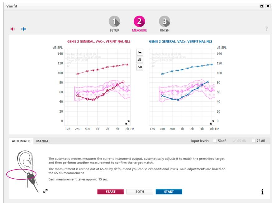
In the **Measure** step, there are two ways of performing verification measurements: Automatic and Manual.
