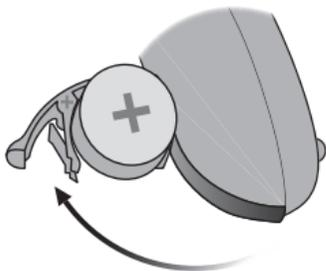
Fully open the battery drawer. Remove the battery.
