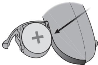
Insert the new battery into the battery drawer. Insert it from above, NOT from the side.
