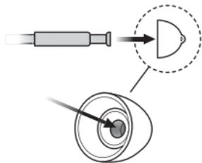
Insert the thin tube exactly into the middle of the earpiece to get a secure fit.
