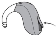
Push the button back into place. You will hear a click when the push-button is closed correctly.
