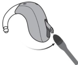
Press the tool into the hole and pull back to open the button door. Ensure you hold the MultiTool as illustrated to avoid damaging it.
