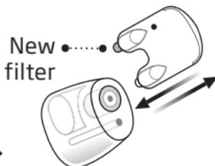
Insert the empty pin into the wax filter in the earpiece and pull it out.
