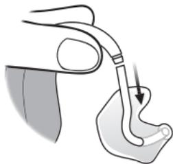
Disconnect the tube and mold from the hook. Hold the hook firmly when pulling it off the tube. Otherwise the hearing aid may be damaged.
