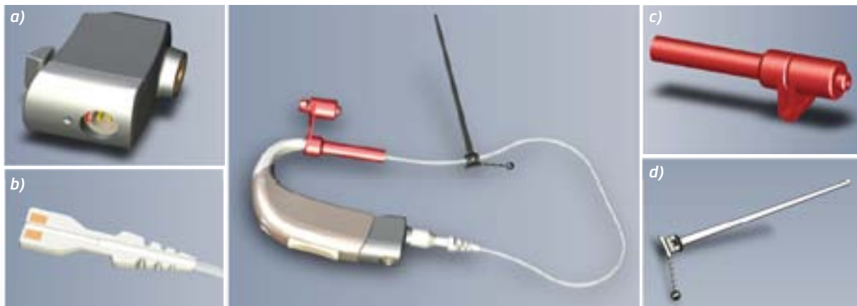
Figure 3: EasyRECD™ tools. EasyRECD™ includes three tools as well as the RECD programming module. The system assembles for calibration as depicted in the illustration (middle). a) A clinically familiar RECD programming shoe interfaces to the bottom of the BTE hearing aid and has the same functionality as the classic Oticon programming shoe. It holds a built-in microphone and magnet for probe tube attachment. b) The EasyRECD™ probe tube has a magnet in one end for attaching it on to the programming shoe. The magnet is covered with silicon which has the effect of creating a perfect seal if a hair should accidentally get caught in the coupling between the probe tube and the RECD shoe. c) The red calibration adaptor is used to assemble the hearing aid and probe tube for calibration. The same adaptor can be used for both BTE and RITE styles. d) The ear strap attaches to the probe tube marking the desired insertion depth in the child's ear canal. The ear strap holds the probe tube in place in the ear of the child. The EasyRECD™ system is not dependent on the ear strap, but the audiologist can use it if he/she finds it helpful. When pulling on the small pin-like structure (bottom, right) the probe tube can be removed without removal of the earmold.
