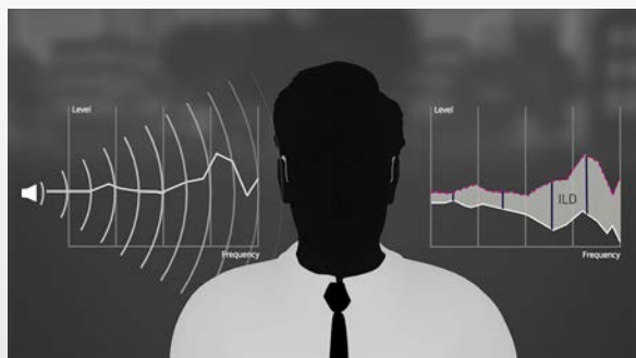
Figure 4: With TwinLink, the number of level estimators have been increased to four for improved ILD precision.
